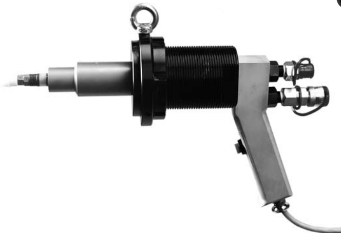
Hydro Expansion Mandrel introduced.
