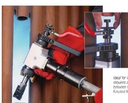
Ideal for limited access areas, the "Wart" MILLHOG® requires a minimum width of 2-3/8" clearance to fit between tubes, and easily clamps into place with the Knurled Knob and Heavy Duty Ratchet.
