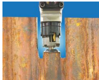
The Standard Mongoose is ideal for end prepping all boiler tube materials and is only 2.25" wide for accessing single tubes in a boiler tube waterwall. It can also be equipped with a membrane removal head for removing membrane from boiler tubes.
