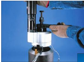
Esco MILLHOG® "Mini" Series end prep tools rigidly mount to the pipe or tube I.D. by a draw rod clamping assembly which centers the tool automatically to produce a clean bevel with a square end.
