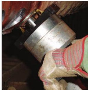
Low RPM and extraordinary torque at the cutting bit make the Mini Millhog a great choice for many tube stub and overlay removal applications.
