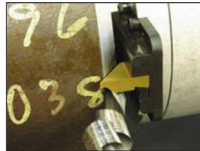
Wide clamp ribs spread the contact force for superior clamping and the Escolock blade locking system minimizes vibration, producing a heavy chip and superior end prep.
