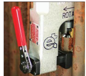
This rugged tool has a narrow profile and fits between 1-1/4" O.D. membrane water wall boiler tubes.
