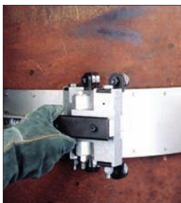
Trolley is adjustable for a variety of EscoWrap Tracks
