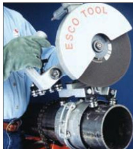
Mount saw to trolley
